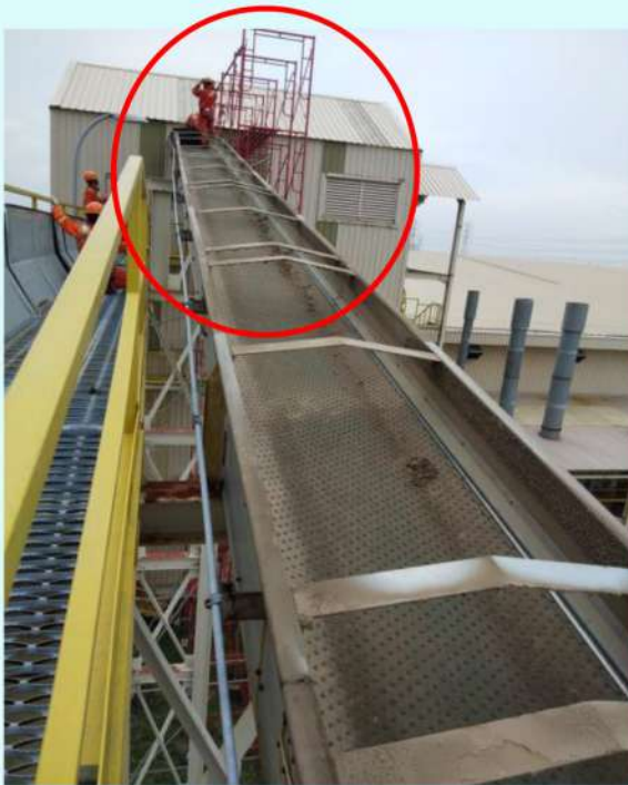
BELT CONVEYOR INCLINE. PANJANG 100 M ELEVASI MAX 26 M
