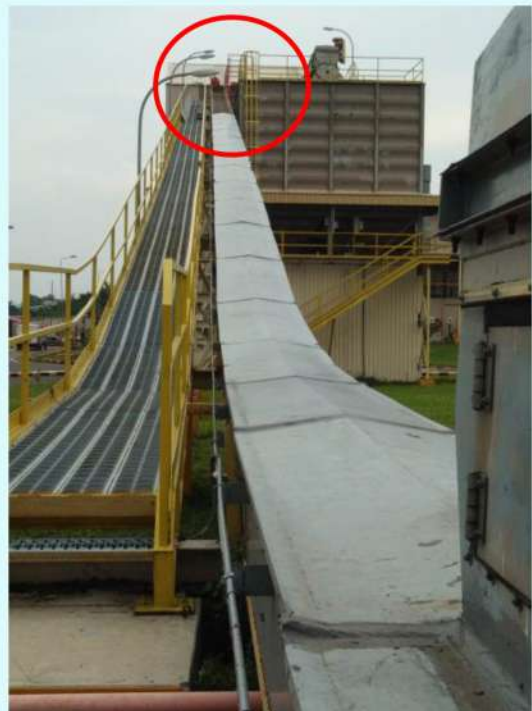
BELT CONVEYOR INCLINE. PANJANG 100 M ELEVASI MAX 26 M
